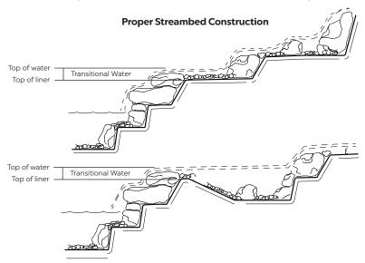
Below is an example of improper streambed construction. Stone, gravel and foam can be combined to make a barrier and create a waterfall, but that barrier will never be watertight. When the pump is turned off, the water will always drain down to the highest point of the liner. Improper construction greatly increases the amount of transitional water.
