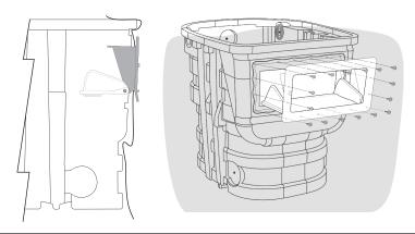
Use your fingers to hold the flange nut and a hand held screwdriver to tighten the screws. The serrations on the flange nut will grab the plastic enclosure once it makes contact, eliminating the need to use a wrench. Use caution when tightening the screws. The screws need only be snug for the silicone to make a seal.
