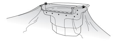
Remove the spring clips and pull the liner away from the face of the enclosure. Make sure that the front of the FilterFalls and the back side of the liner are clean and free of debris. Apply a full, continuous bead of Atlantic fish-safe RTV silicone to the face of the FilterFalls along the center line of the threaded inserts.
