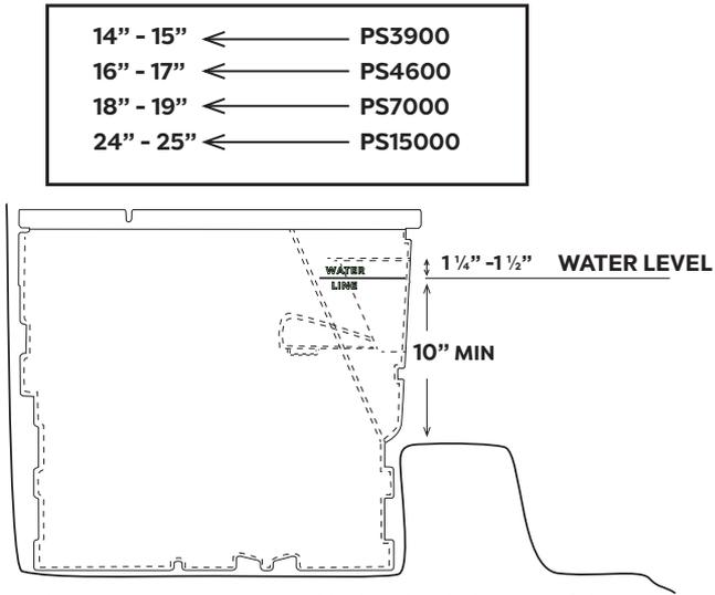
Place the Skimmer enclosure into the excavated hole. Check the top of the enclosure to make sure that it is level front-to-back and side-to-side. Check where your pre-determined water level falls on the face of the Skimmer enclosure. The water level needs to be between 1/4" and 1/2" below the top of the weir door opening and/or even with the water level indicator molded on the side of the Skimmer.
