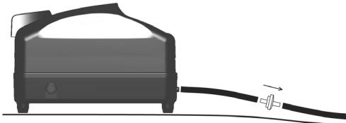
Note: The outlet side of the check valve has a small "OUT" molded in the side. Direction of flow can be easily verified by blowing into the end of the check valve.
