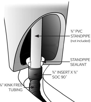
Atlantic's FB3200/FB4600 Fountain Basins have a recessed pocket that allows 1 $\frac{1}{2}$ " conduit sleeves to be installed within the circumference of the basin without notching for the pump cord and low voltage wiring. A 1 $\frac{1}{2}$ " cord stopper is included to plug the top of the sleeve to prevent gravel and other debris from entering the conduit.
